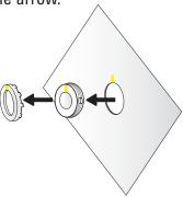
**4. Find the Notch:** Push the connecting rod all the way down through the orange o-ring. Then gently pull back up on the connecting rod until you feel the groove seat into the o-ring.
