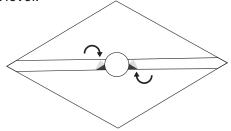
**2. Activator Rolling:** Roll the activator at an angle around the activator frame. This allows for a tighter roll, making it easier to push through the drilled hole.
