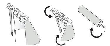
**3.** Align the Three Yellows: When fastening the nut, align the yellow paint on the activator frame to the arrow on the sticker. The nut also has yellow paint to align with the arrow.
